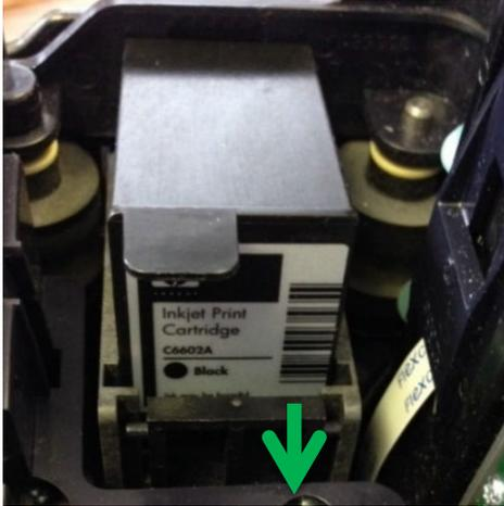
3. Pull the inkjet cartridge out of the scanner.
