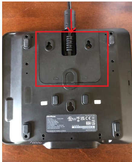
Figure 4. Insert the I/O (input/output) Block into the Back of the Verifone M440 Terminal
