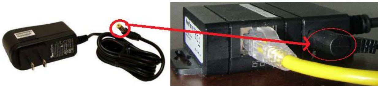
Figure 2. Plug Power Adapter into the I/O Block
