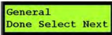
(4) The CAD will then display the first diagnostic group name, i.e., “General”. Press the right (NEXT) button until the desired diagnostic group is displayed (see the CAD “Diagnostic Menu” in the graphic above for the diagnostic group names).
